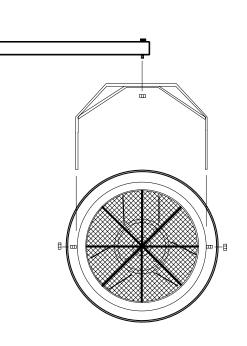
6. Check fan rotation upon startup. Standing in front of fan, the blade should be turning clockwise. If rotation needs to be reversed this usually can be accomplished by reversing the connection wires.
